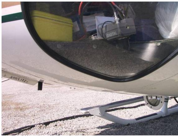
Figure 7. Digital video camera typical mounting location.
