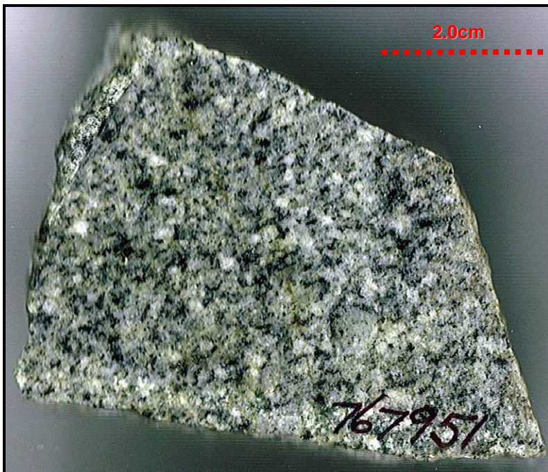
PLATE 3: Granodiorite: Sample # 767951 - Leucocratic to mesocratic, fine grained equigranular matrix with local euhedral plagioclase megacrysts (up to 7mm measured), trace very fine grained disseminated pyrite.
