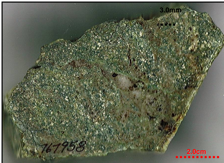
PLATE 16: Andesite Lapilli Tuff: Grab sample# 767958 - Light green, massive looking outcrop supporting fine grained clasts dominantly with minor coarse grained fragments
