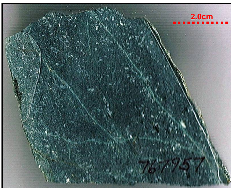
PLATE 14: Andesite Lapilli Tuff + Basalt Dyke: Outcrop grab sample# 767957, trace to 0.5% very fine grained pyrite disseminations and fracture fill.
