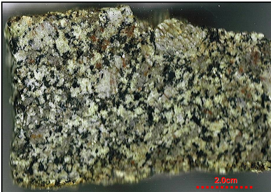
PLATE 5: Granodiorite: Sample# 767952 - Leucocratic to mesocratic, fine grained equigranular matrix with local euhedral plagioclase megacrysts (up to 1- 1.5cm measured)
