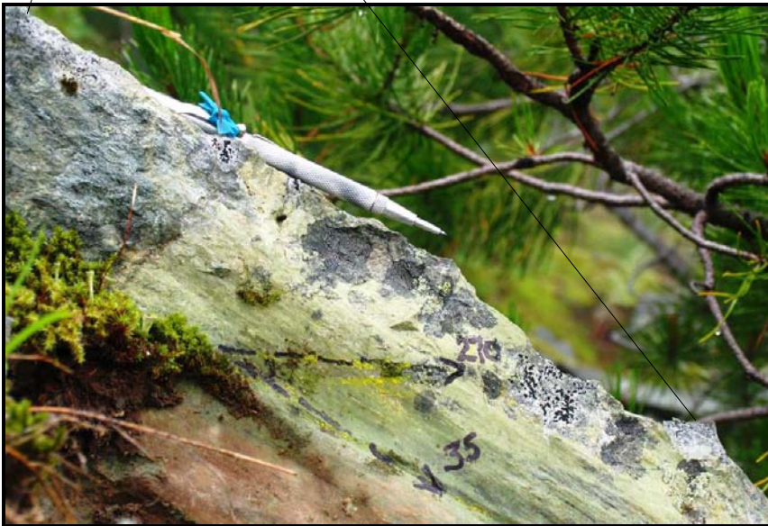
PLATE 13: Andesite Lapilli Tuff + Basalt Dyke: Outcrop grab sample# 767957 – Slickened-serpentinized surface with possible reverse movement noted. Bedding measured = S0 @ 120/60. Slickenside measured @ 35-->270
