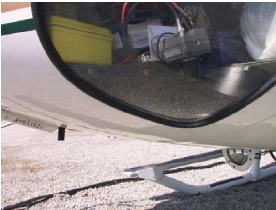
Figure 6. Digital video camera typical mounting location.
