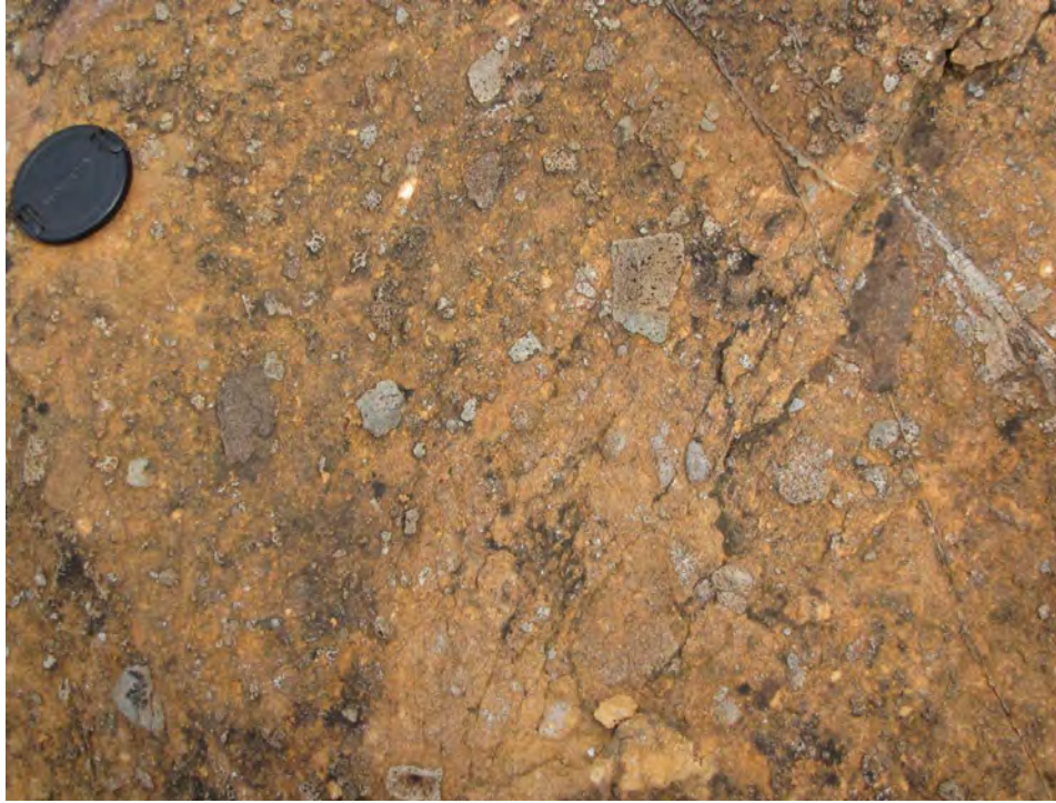
Figure 7. Detail showing pervasively Fe carbonate altered matrix to mafic fine- to medium-grained lithic lapilli tuff, probably of Upper Triassic Stuhini Group; Inlaw Creek area.
