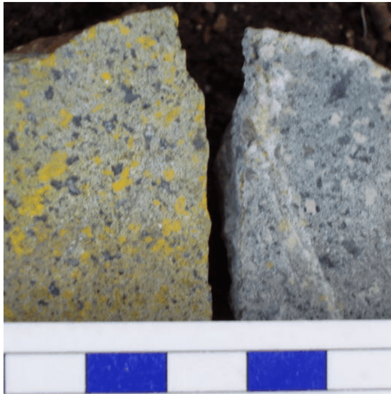
Figure 8. Stained (left) and etched (right) slabs of hornblende(?) - pyroxene feldspar bearing fine- to medium-grained monzonite or monzodiorite; bars at base are 1 cm.
