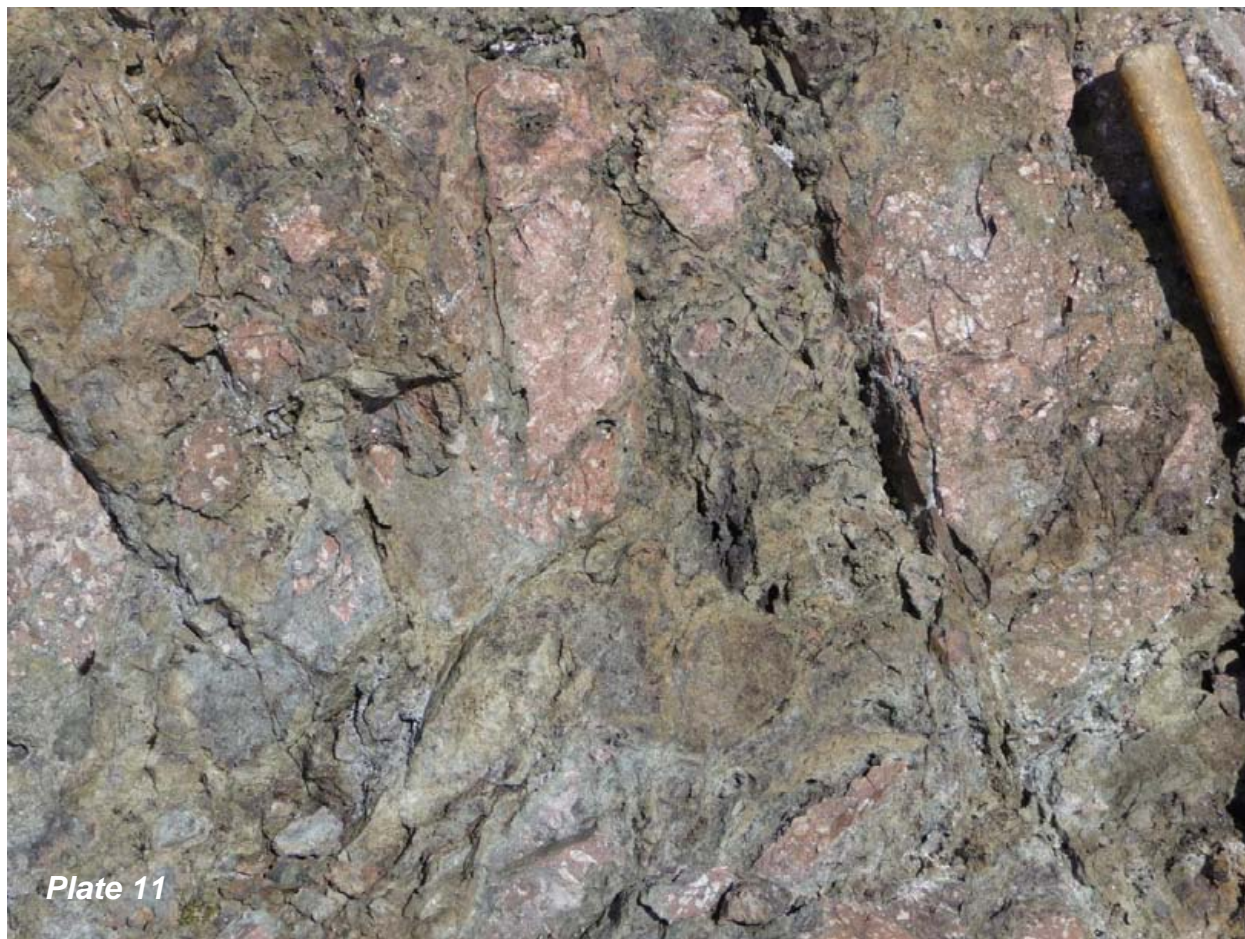
Plate 11: Skarn-cemented Breccia with Syenite Intrusive Clasts
