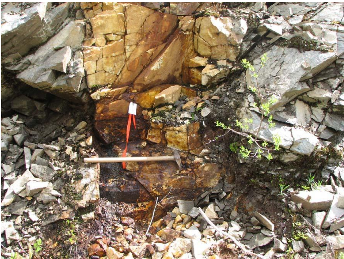
Highly mineralised Quartz Vein – La Forme Creek Road Mineralisation consists of massive Pyrrhotite with minor Chalcopyrite
