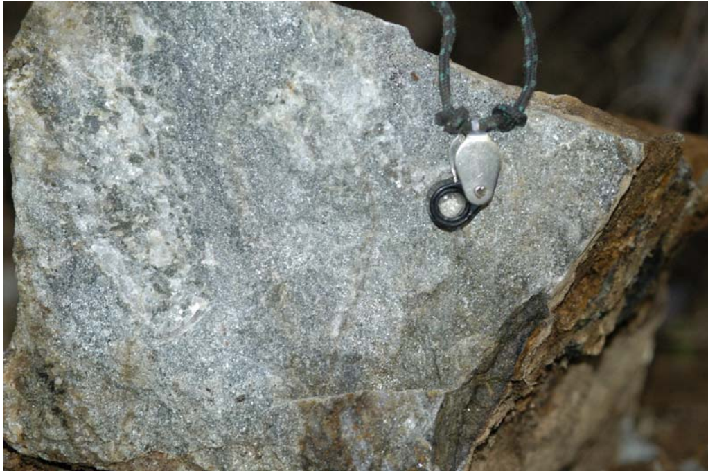
Figure 8: Bedrock exposed in hand-dug trench: quartzite, pelitic quartzite and slightly calcareous quartzite having disseminated pyrite and highly reflective graphite.
