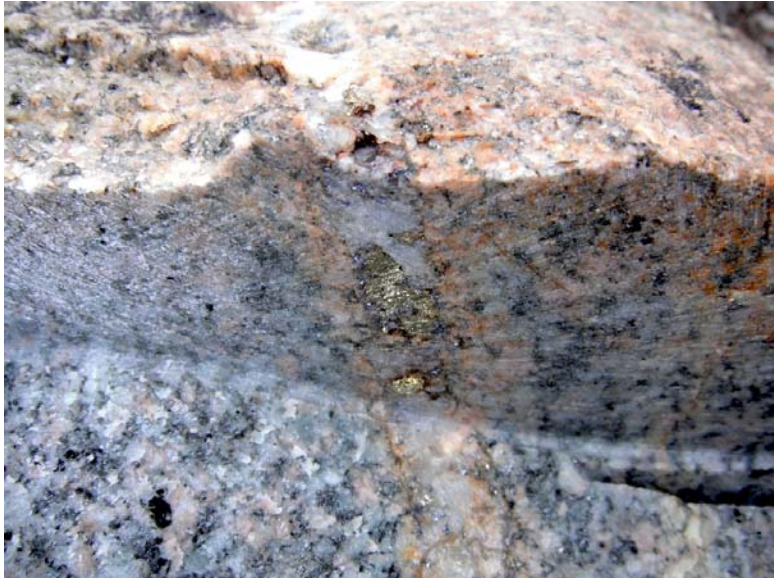
Plate 11: Channel sample showing quartz-sulphide veins leached at surface.
