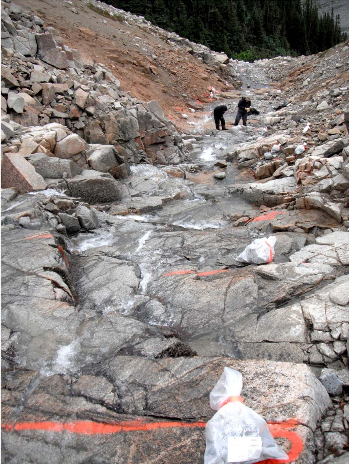
Plate 10: Channel sampling included fifty-nine 2m samples and one 3m sample.
