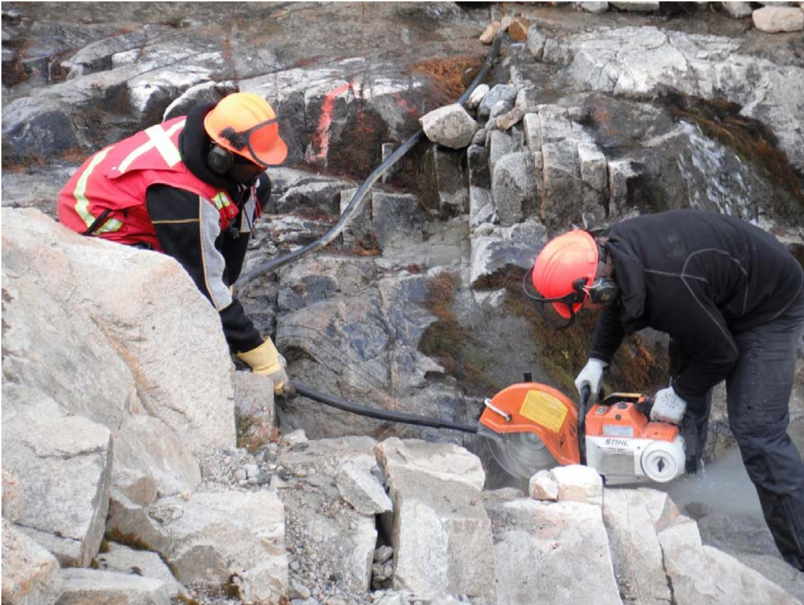
Plate 8: A portable rock saw used to sample mineralization at Troitsa Main.
