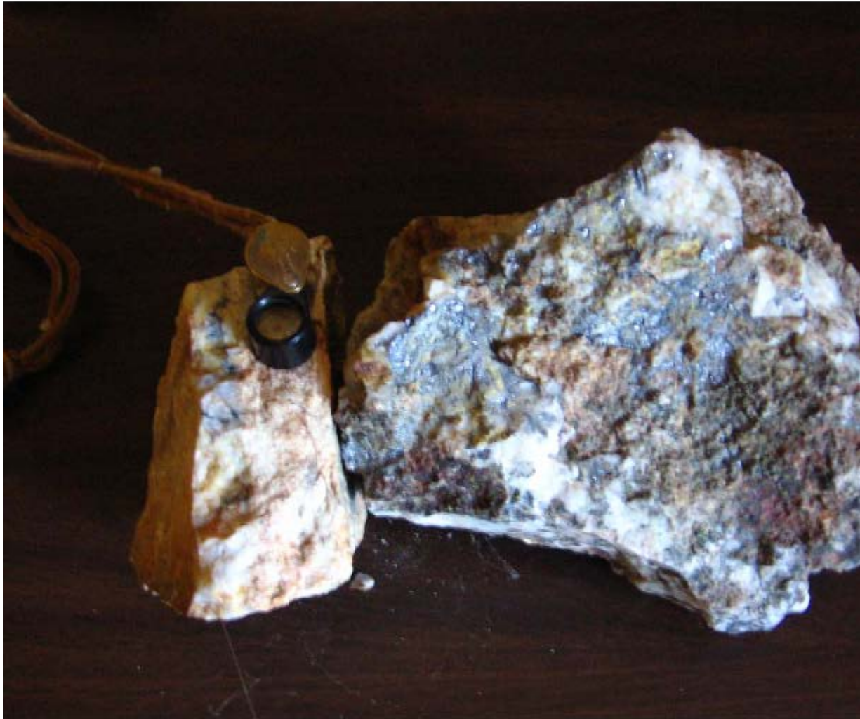
Rice Creek Mo Zone: Samples of molybdenite mineralization collected along the talus slope of the Quartz Monzonite intrusion (see accompanying photos). Moly is mostly associated with the quartz veins and disseminated arsenopyrite. Some of the veins are anomalous in gold.
