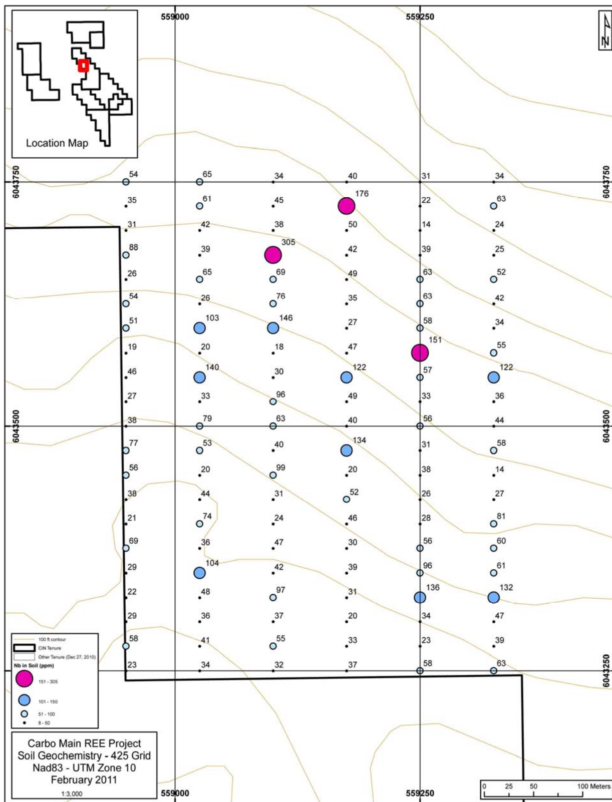
Figure 8. Carbo Property Soil Sampling – 425 Grid – Nb
