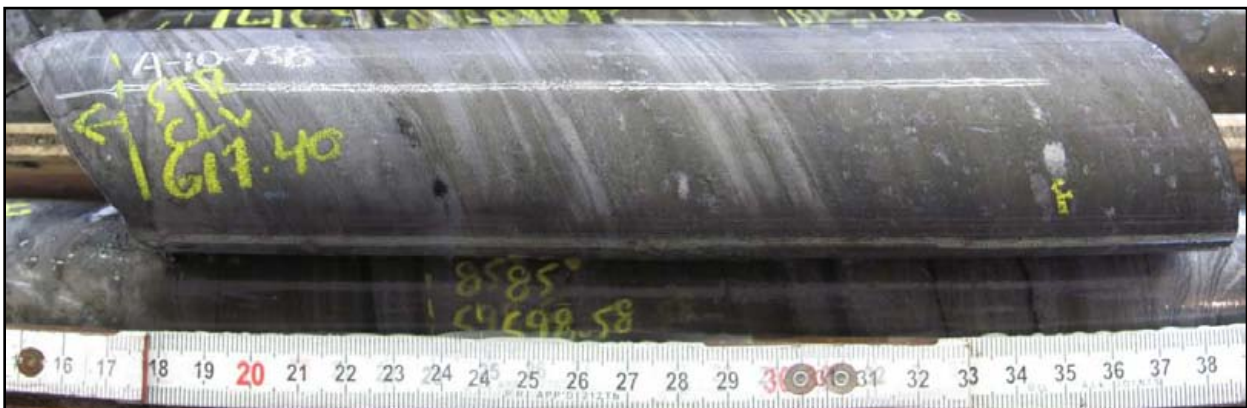
Plate 5: High grade Sp mineralisation displaying mottled texture interbedded with granular Ba beds in A-10-73B @ 617.40m.
