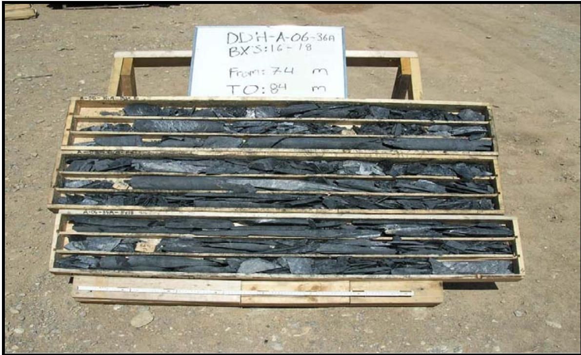
Plate 11: Intensity of cleavage, Hole A-06-36A boxes 16-18.
