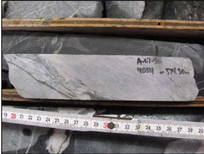
Plate 6: Massive granular barite bed with minor pyrite (brown) in A-07-50 @574.30m.
