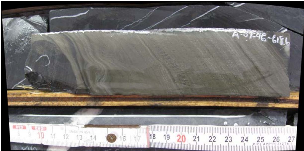
Plate 3: Bedded Py with minor sphalerite bands within Proximal Facies from A-07-46 @ 618.60m. Laminated Rip-up clast present on the left side of the drill core.
