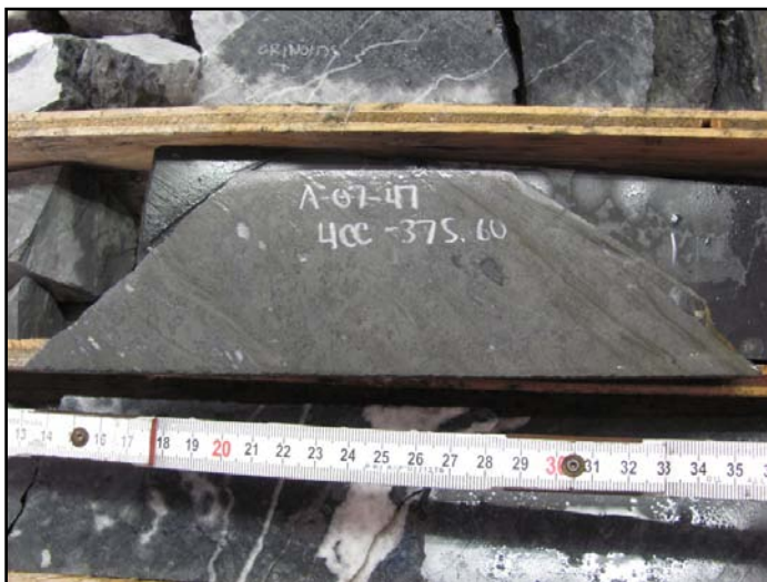
Plate 4: High grade sphalerite mineralisation displaying “Mottled” texture in Cardiac Creek Zone facies in A-07-47 @ 375.60.
