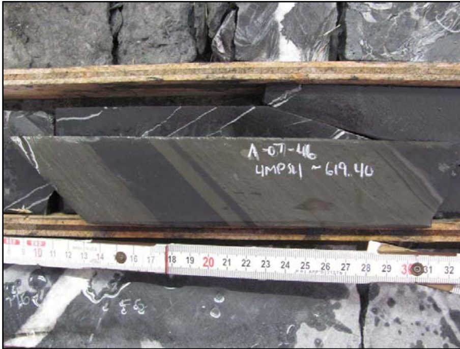
Plate 2: Interbedded Py and shale representative of the Proximal Facies in A-07-46 @619.40m.
