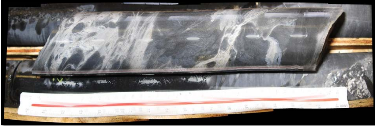
Plate 8: Sphalerite-rich sulphide breccia in Road River rocks in A-08-63 @ 479m.
