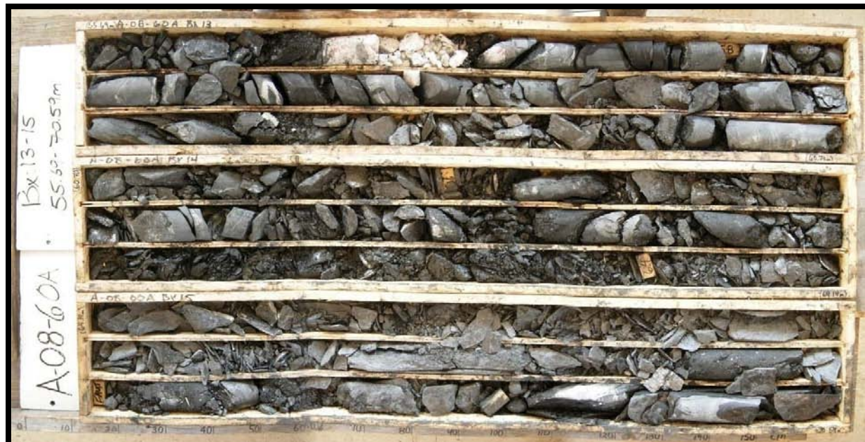
Plate 12: Bad ground associated with brittle faulting, A-08-60A Boxes 13 to 15.
