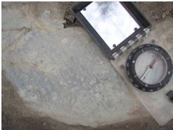
Figure 24: striae on flat outcrop indicating ice flow towards 305^{\circ} ; note – smooth and abraded surfaces facing in the up-ice direction (bottom of photo) versus broken fractures facing down-ice (top of photo).
