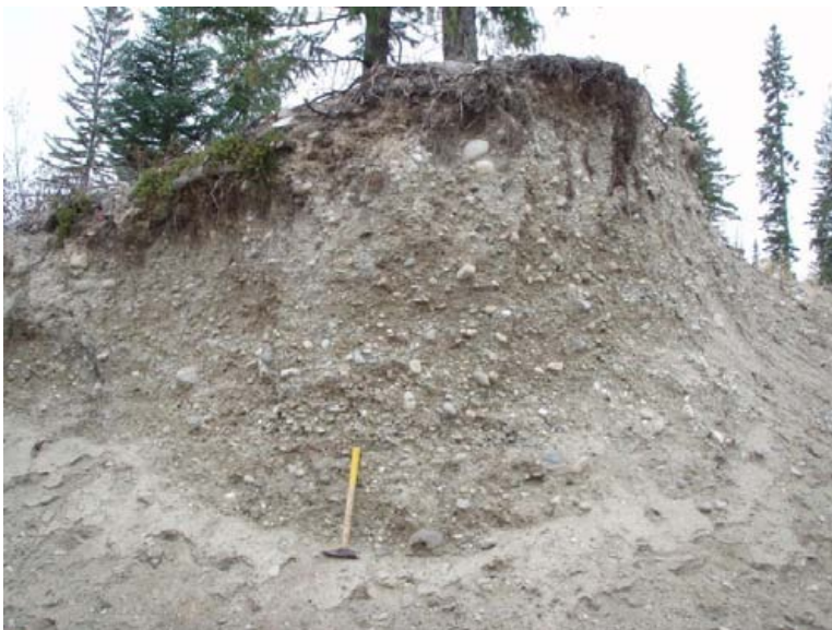
Figure 3: sandy diamict and interbedded gravels exposed in a small hill in hummocky moraine (Mh)
