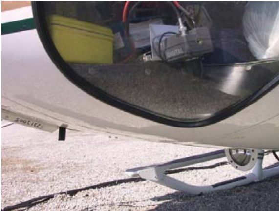
Figure 6. Digital video camera typical mounting location.
