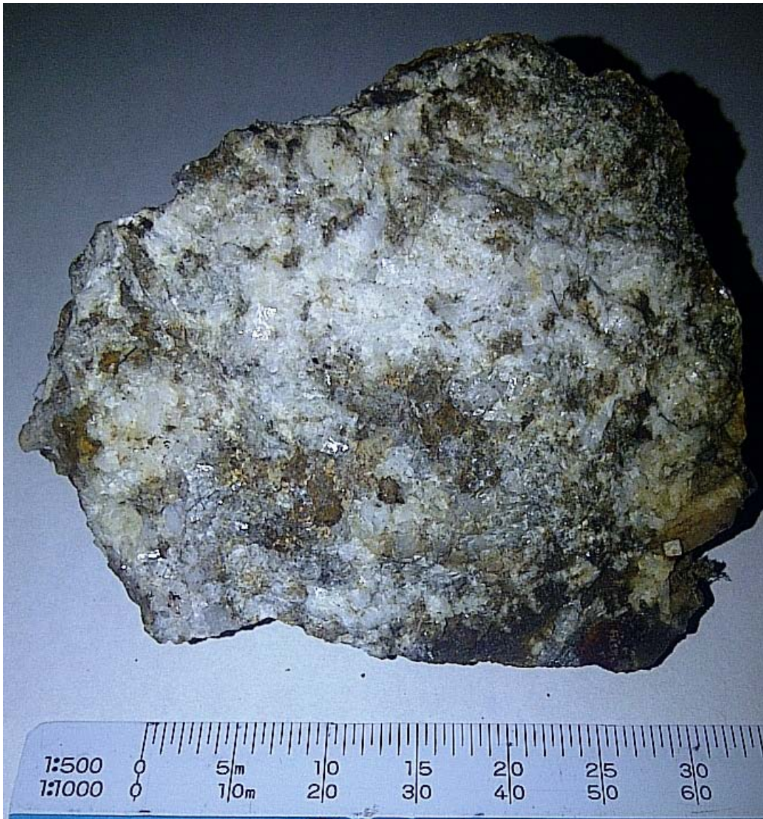
ROCK AW11-01 – 307165 E 5654632 N Float Feldspathic endoskarn. 75% feldspar, 10% quartz remainder green chloritized mafic. Located northeast of 1W 0N old steep grid. 10M ON SCALE =1 CM
