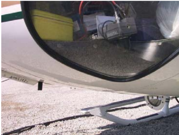
Figure 6. Digital video camera typical mounting location.
