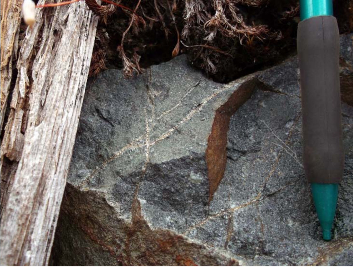
Image No. 2 Pyrite filled fractures of stockwork-like veining in propylitic altered basalt.
