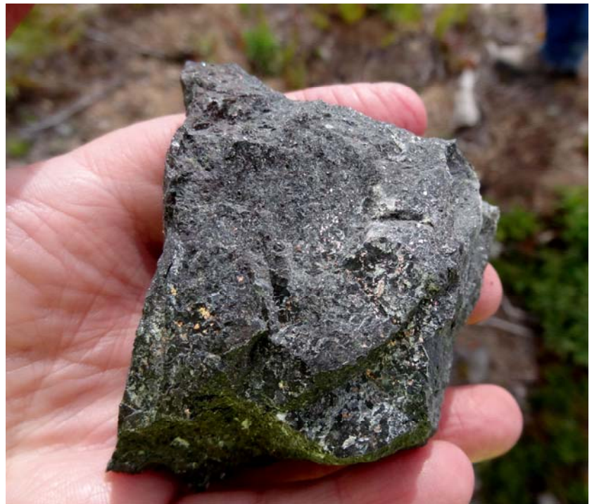
Photo 5: Specimen from the Native Copper Showing. Foil-like flecks up to a few millimeters across pepper the hard, weakly altered to unaltered basaltic tuff.
