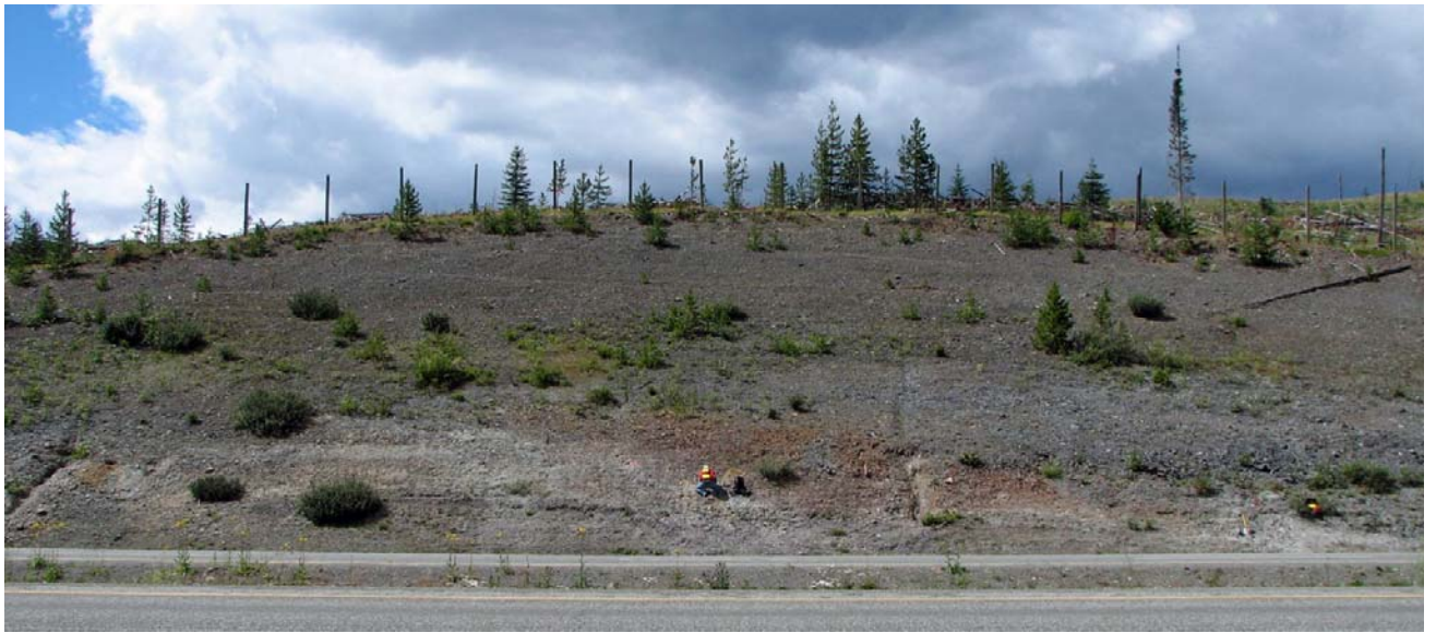
Photo 2: Sampling at the Blacktop Showing in 2007. Looking due west across both lanes of the Coquihalla Highway. Some of the reopened trenches that were sampled are clearly visible. Note the rusty patch of subcrop of the hangingwall andesites (Unit 3) and the lighter, buff colored sericitic subcrop (Unit 2) that hosts the mineralization.
