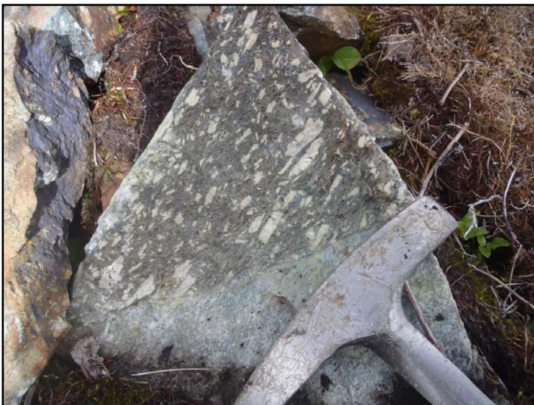
Photo 10. Elongations of feldspars crystals defining foliation seen in station BC11SS074 (Appendix 1).
