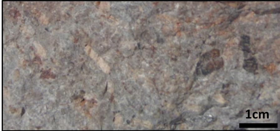
**Photo 5. Crowded feldspar porphyry in hand specimen**
