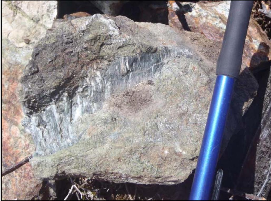
**Photo 9. Actinolite-quartz-epidote veins at station BC11SS070 (Appendix 1)**
