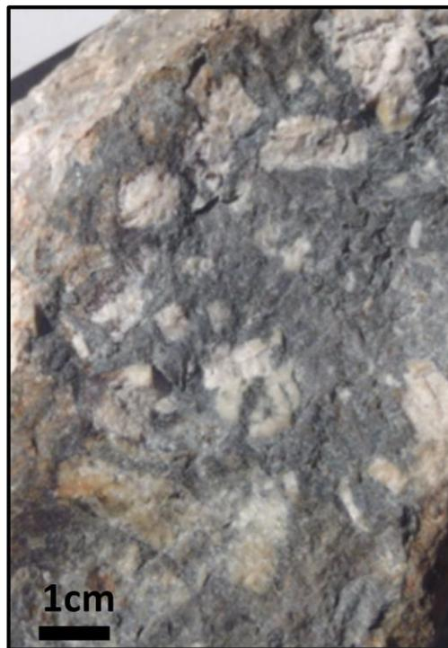
**Photo 2. Megacrystic plagioclase and hornblende-phyric diorite hand specimen**
