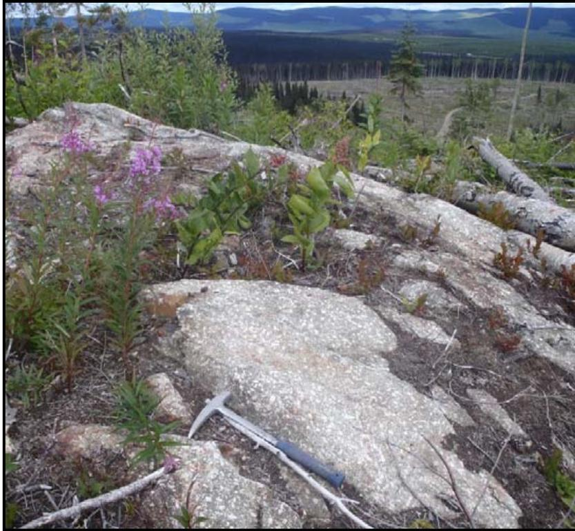
**Photo 1. Megacrystic plagioclase and hornblende-phyric diorite in outcrop**
