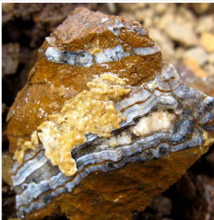
ABOVE. WP164 . Crustiform quartz, and colloform chalcidony (after opal). Late coarse calcite fill.
