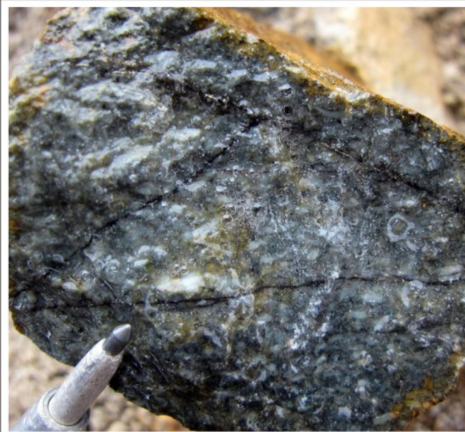
ABOVE. WP 180 [410586 6350773]. Secondary biotite veinlets. This indicates porphyry-type alteration (potassic).
