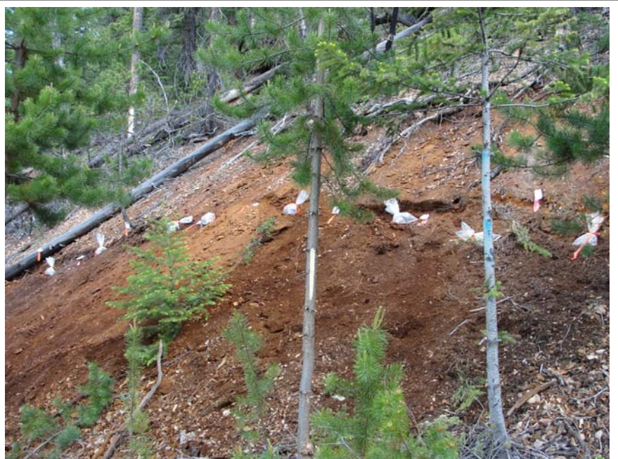
Photo 4: Sampling the Ferricrete Zone. View looking west of the rusty weathering talus and the series of eight 1m-long samples cut through it.
