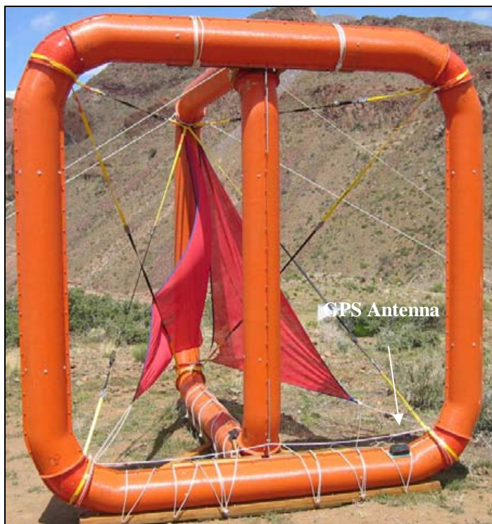
Figure 5 - ZTEM base station receiver coils.
