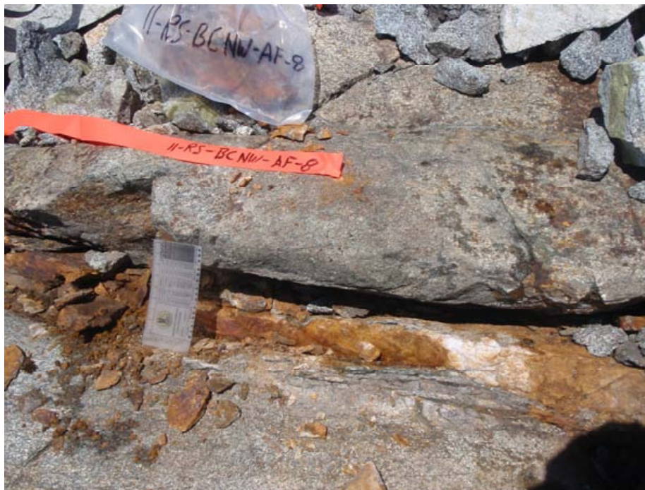
Figure 7: Mesocratic tonalite with a rusted quartz vein, with a grain size card for scale; sample 11-RS-BSNW-AF-08.
