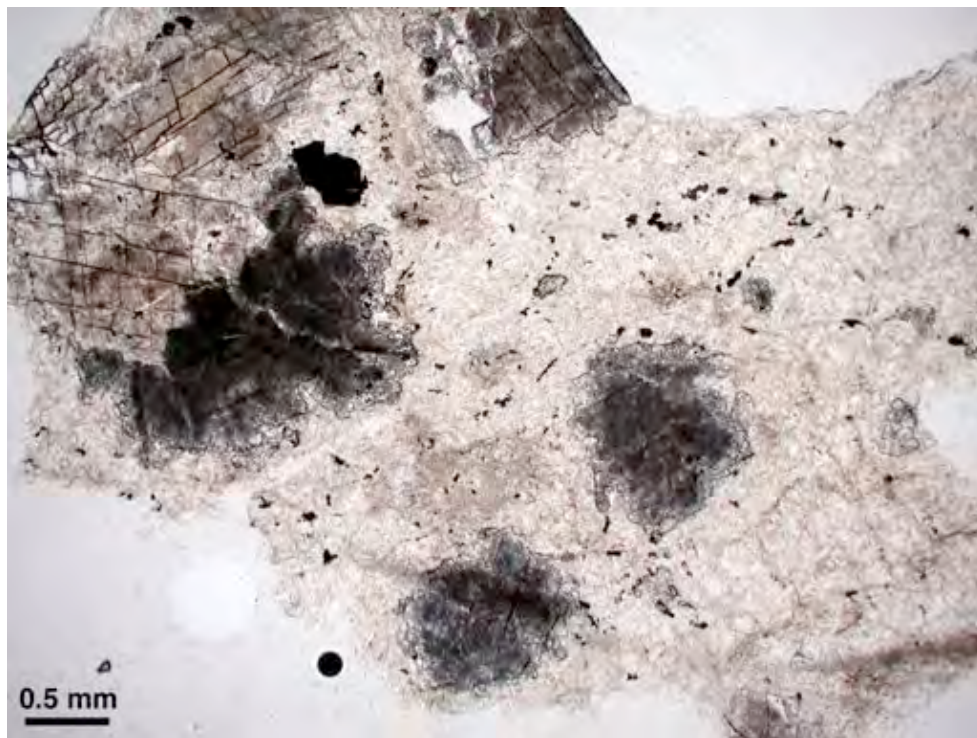
Figure 3c-1: two generations of carbonate (older: darker, inclusions rich; younger: coarser, clearer) overprinting talc fragment with opaque inclusions. F.o.V. 4.5 x 6.00 mm, PPL.
