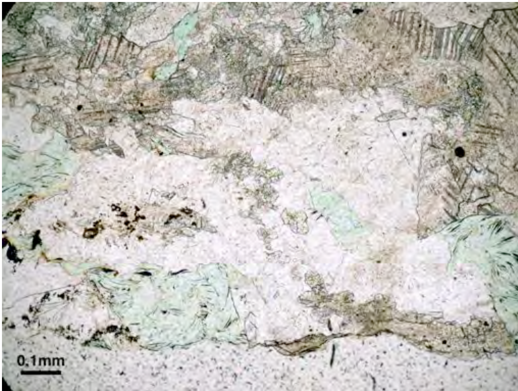
Figure 3b-2: pale green Cr-muscovite intergrown with quartz and carbonate. F.o.v. 0.97x 1.30 mm, PPL.
