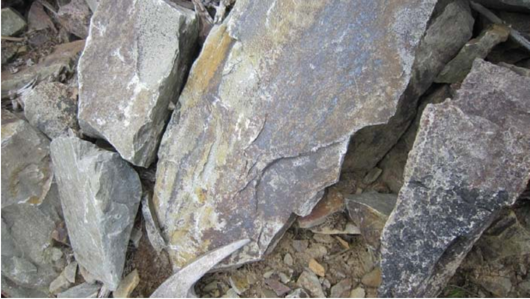
Photo 3: Fracture controlled hematite and manganese oxide (pyrolusite?), also within bleached (argillic altered) siltstone; this alteration is less intense than is shown in Photo 2.
