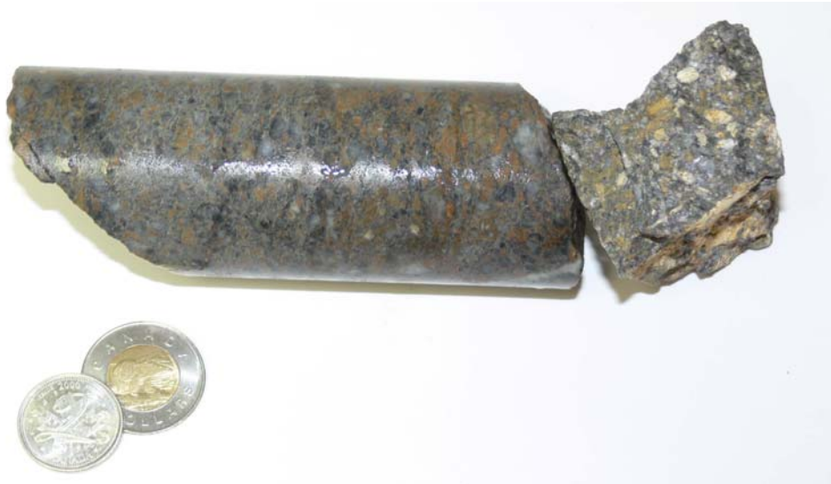
Plate No. 1. 'Blue-quartz-eye schist'. Core on left is from 2004's DDH hole FC04-13 approximately 400 m north of the 2007-2008 trenching area (F9 Area). Rock on right is float from the Discovery Trench area. Both are less altered and foliated versions of the quartz muscovite schist associated with massive sulphide lenses in the F9 Area. The rock is characterized by pale milky blue quartz 'eyes' thought to be rounded phenocrysts in a rhyolitic volcanoclastic; some 'eyes' are subhedral with straight sides. A blue quartz 'eye' is seen in the core just above the line of the light glare. Brown areas on the core appear to be Fe carbonate. White spots in the rock on right have straight sides and appear to be feldspar phenocrysts, relatively rare in the schists.
