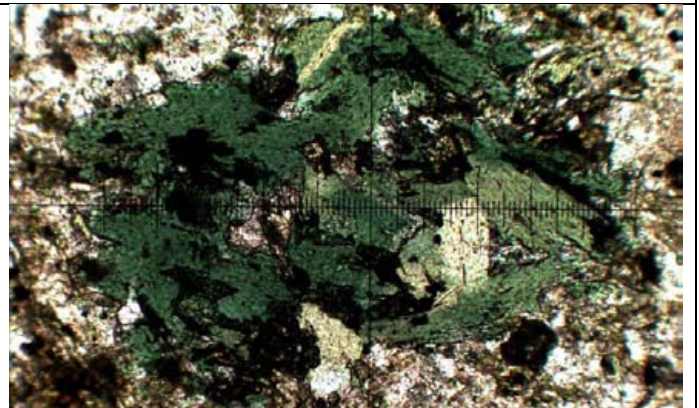
E. Photomicrograph showing chlorite. PPL. FOV is 0.8 mm.
