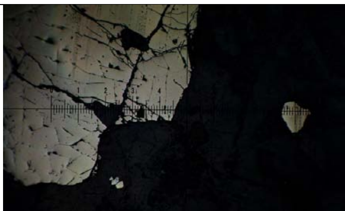
D. Photomicrograph showing pyrite grain. RL. FOV is 0.8mm.
