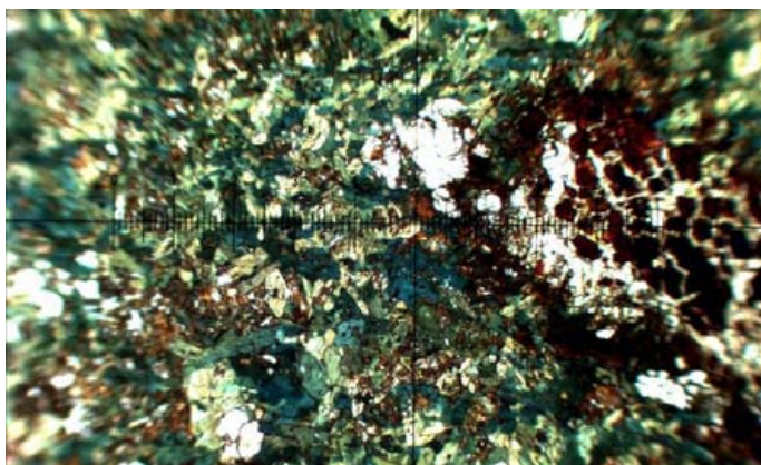
C. Photomicrograph showing chlorite alteration. PPL. Field of view is 2mm across.
