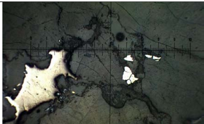
E. Photomicrograph showing silver. RL. FOV is 2 mm.
