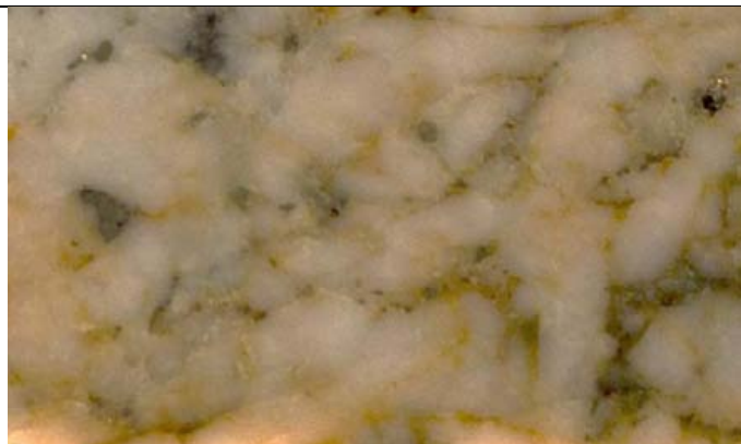
B. Prepared section off-cut. Field of view is approximately 25mm x 40 mm
