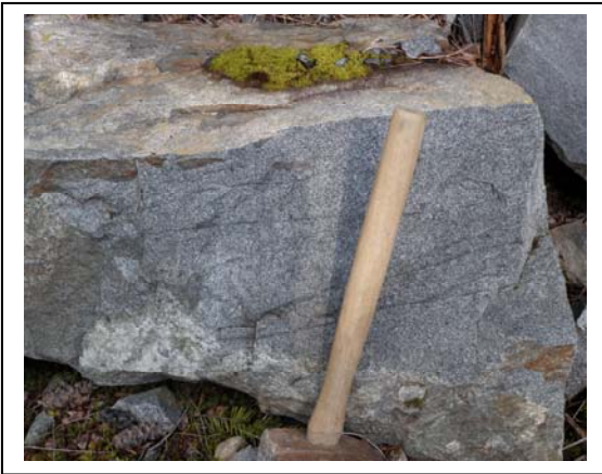
Photo 4: Site #3 disseminated pyrite-magnetite in quartz-epidote veinlets in diorite
