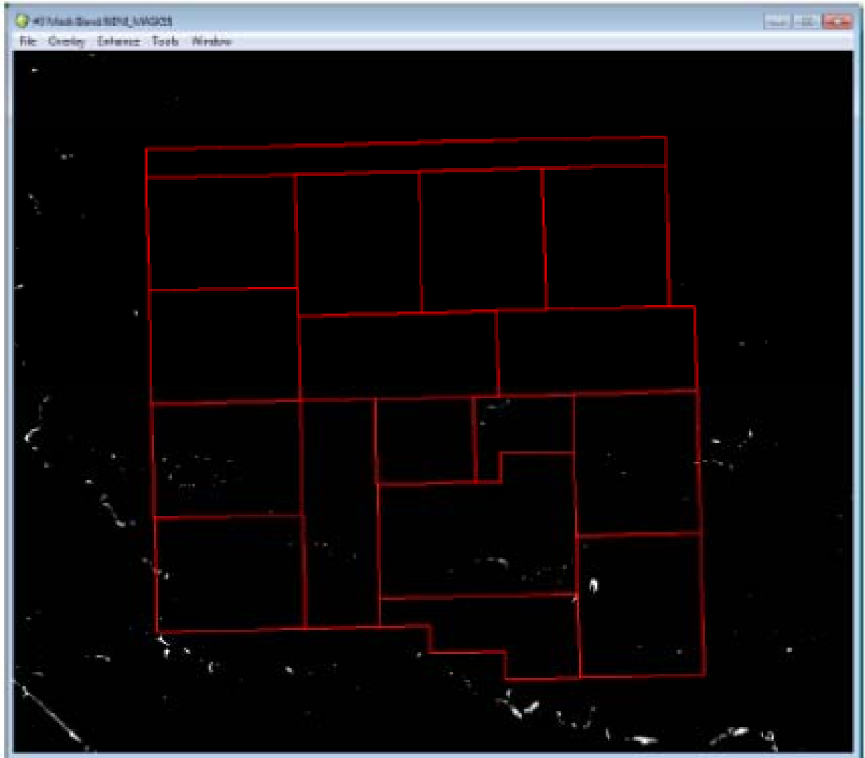
Figure 6: Mask (black) removing from analysis calculation areas presenting no useful bedrock data. Note the general lack of mappable pixels within the property (Kilby, 2011).
