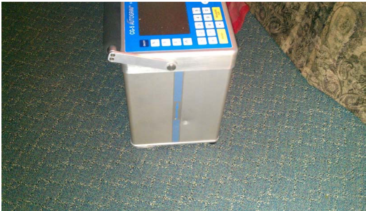
Photo 9: The external damage to the CG-5 Autograv.
