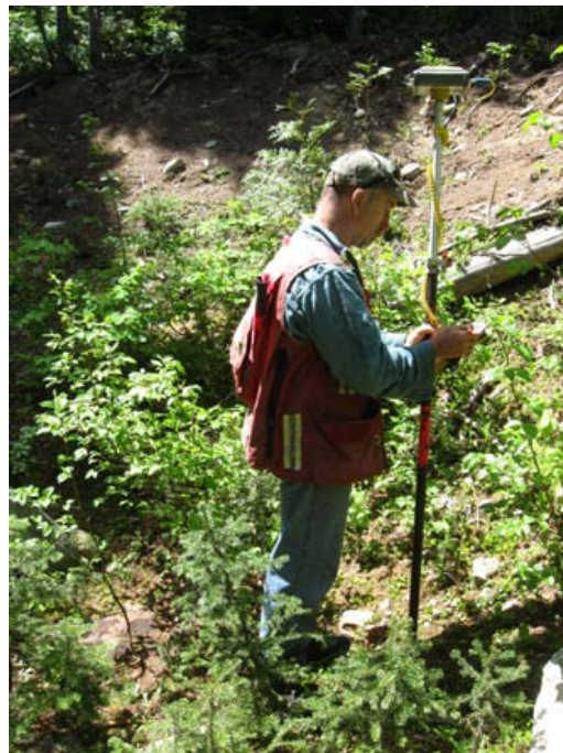
PLATE 4: GPS rover collecting collar XYZ data.
