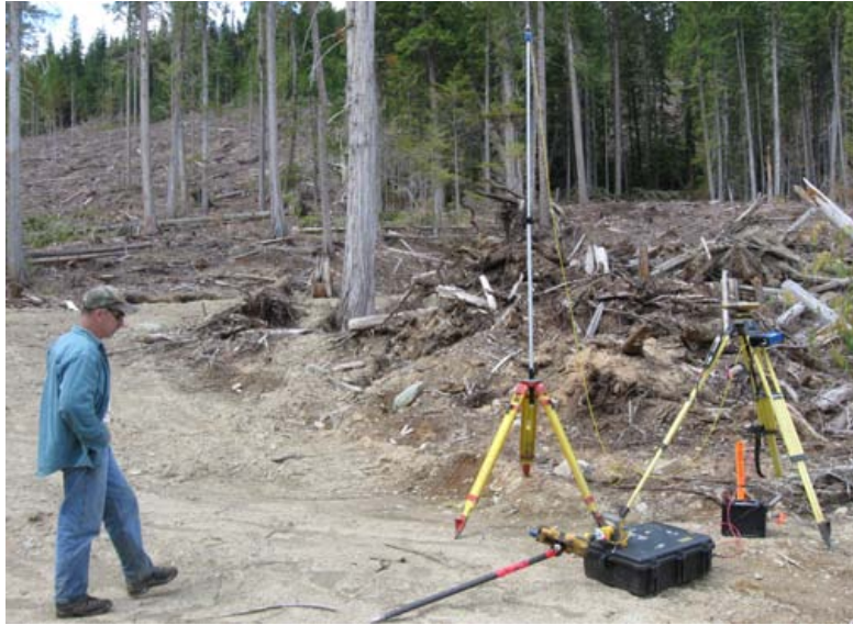
PLATE 2: July 2011, Topcon Legacy-E RTK GPS system (base station and RTK rover) positioned on the Swift Katie property. Devices are owned and operated by SEL Survey and Design located in Nelson BC.
