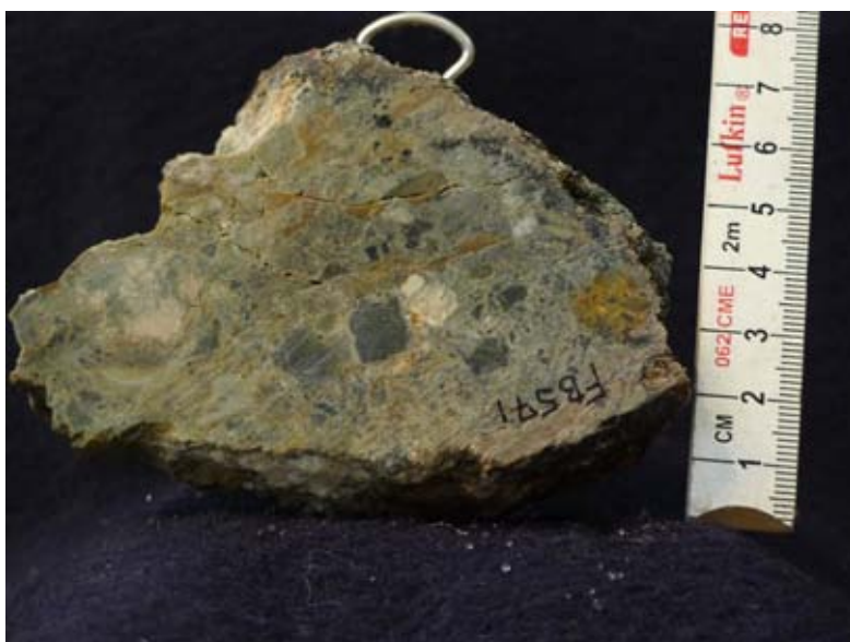
Photo Plate 3. Epiclastic rhyolite breccia or volcanic conglomerate. Matrix-supported angular to subangular clasts display varying coloration and alteration styles. Pale bleached, darker chlorite-altered, and rusty oxidized fragments are prominent.
