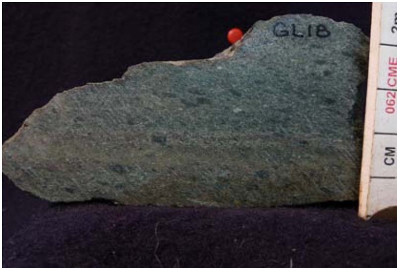
Photo Plate 12. Macro photo of banded, intermediate tuffaceous lapilli and pebble sandstone from the lower series tuffaceous stratigraphy.
