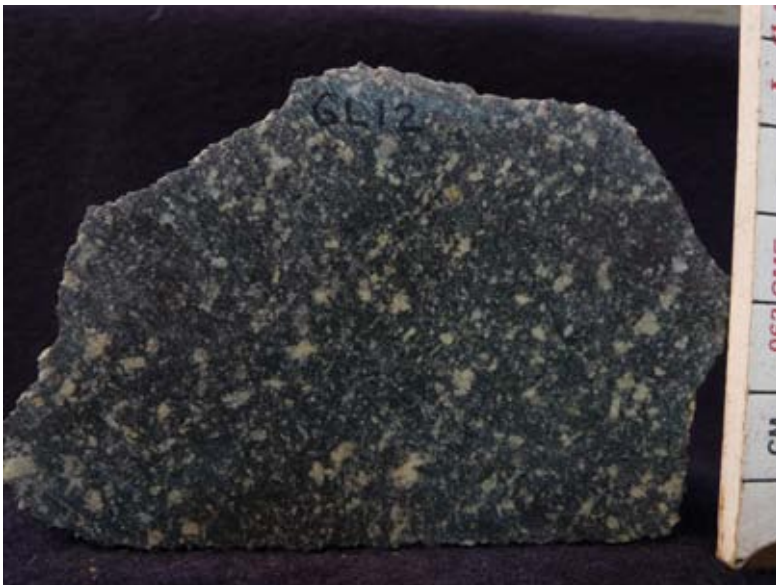
Photo Plate 13. Medium-grained hornblende-feldspar-porphyrific intermediate intrusive rock. These rocks form sill like bodies within the lower series tuffaceous stratigraphy. Sample displays weak chlorite alteration.
