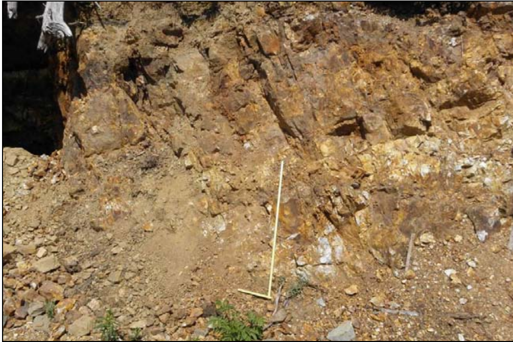
Figure 8-1: International Vein (with one metre scale) The vein is quartz with irregular massive sulphide bodies of galena, pyrite, and rare sphalerite.
