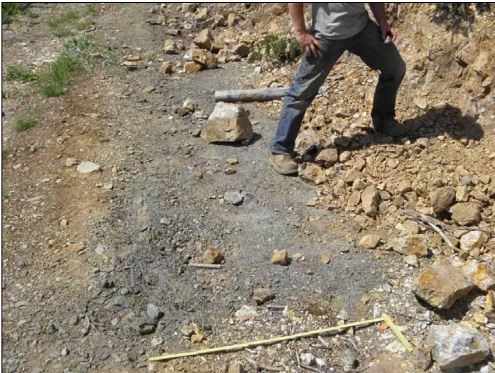
Figure 8-2: Black, Carbonaceous Schist, in the Footwall of the International Vein (with one metre scale)
