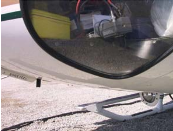
Figure 7. Digital video camera typical mounting location.
