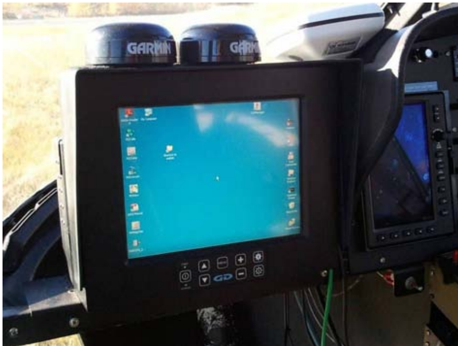
Figure 6: AGIS installed in the Eurocopter AS350.
