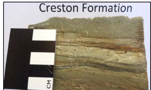
6b. Green laminated Creston Formation: fine to very fine sandstone, siltstone, and phyllite
