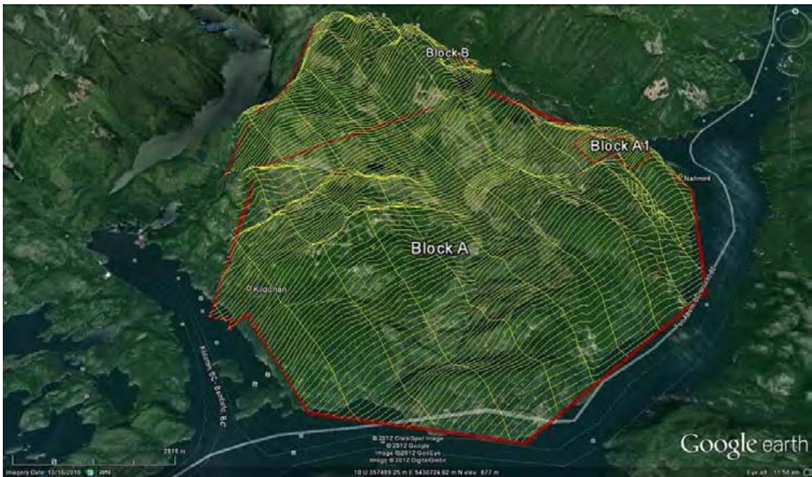
Figure 5: Terrain View – Block A and Block B with survey and tie lines outlined in yellow and the boundary in red.
