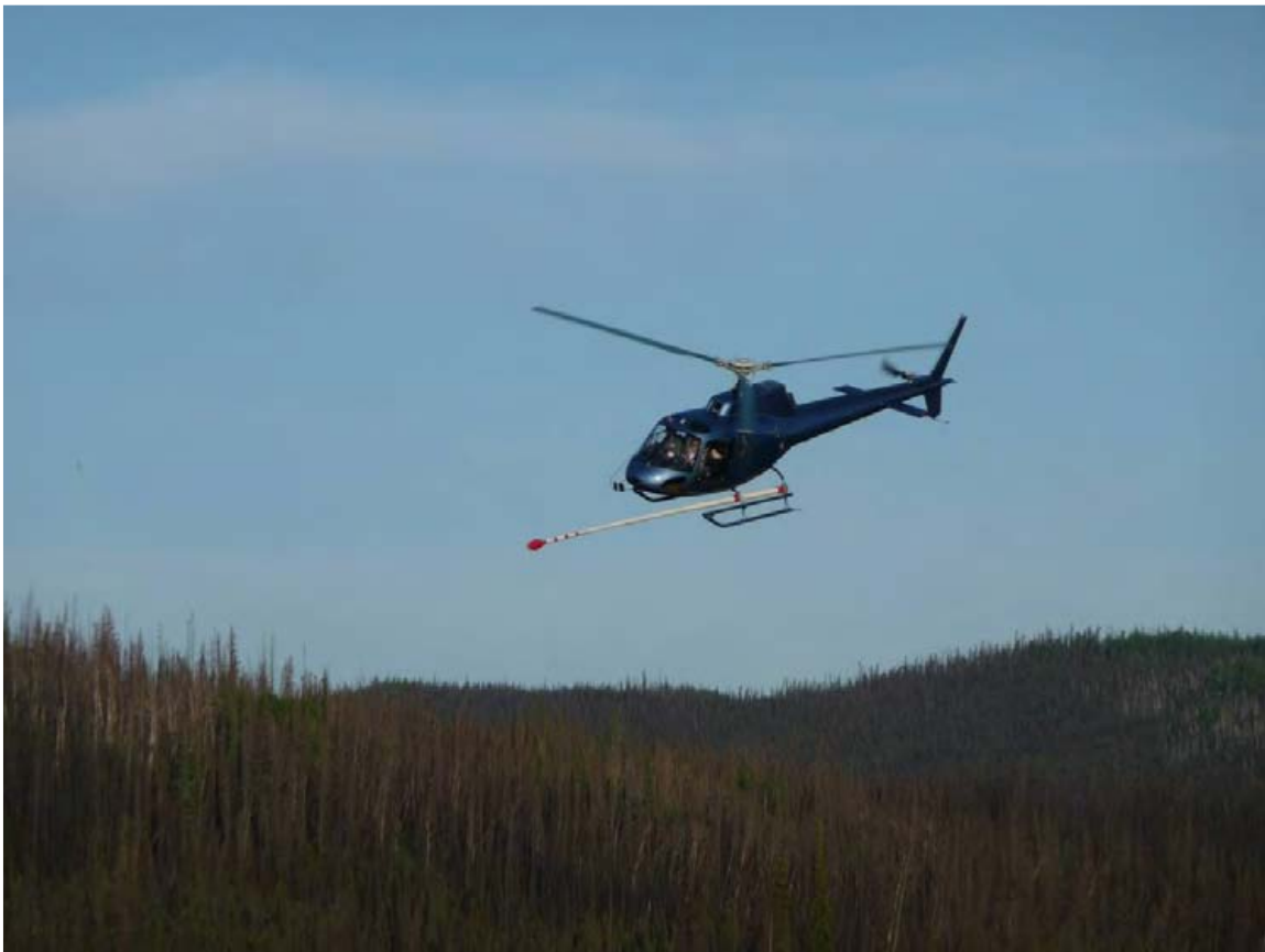
Figure 9: Eurocopter AS350 equipped with mag stinger for magnetic data acquisition.
