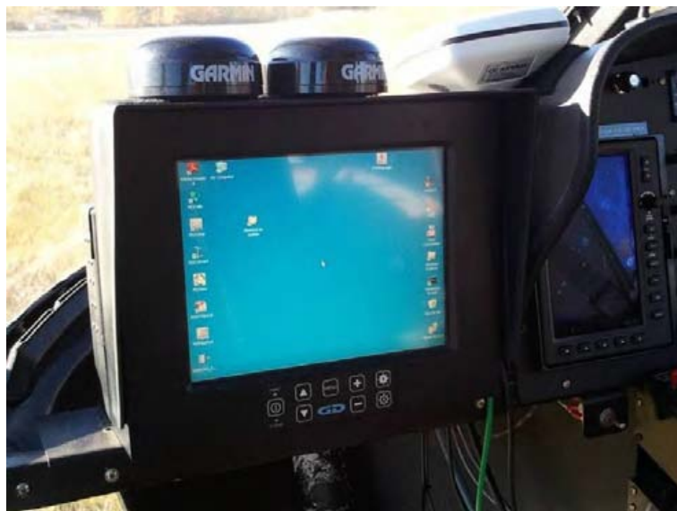
Figure 10: AGIS installed in the Eurocopter AS350.
