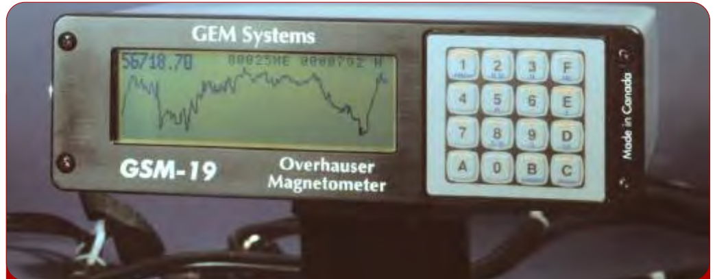
Overhauser (GSM-19) console with sensor and cable. Can also be configured with additional sensor for gradiometer (simultaneous) readings.
