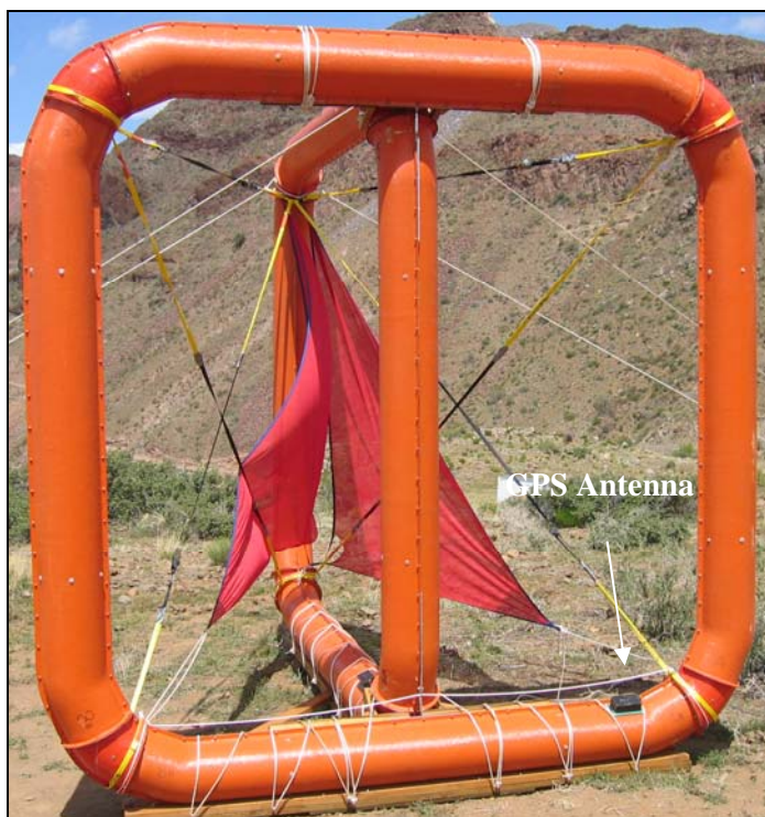
Figure 5 - ZTEM base station receiver coils.
