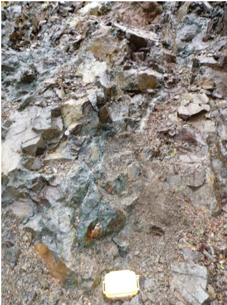
Photo 9: October 10, 2011: main showing; malachite- stained massive sulphide lense
