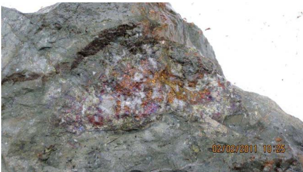
Photo 2: quartz-pyrite-chalcopyrite-bornite pod (blow-out)
