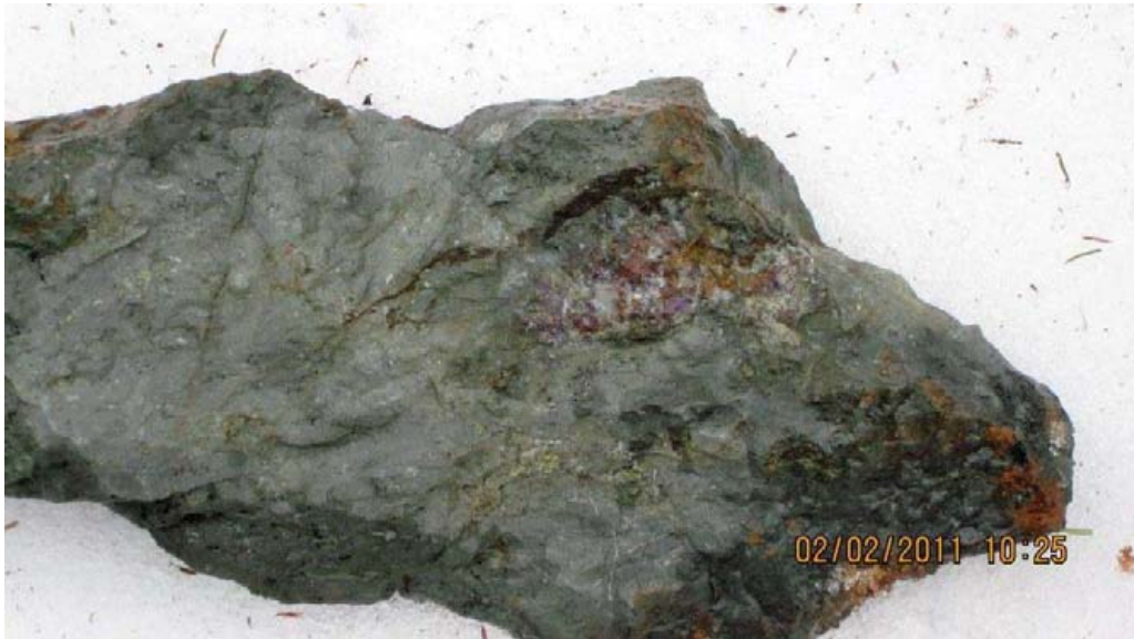
Photo 1: epidote-calcite-quartz stringers through basalt with quartz-pyrite-chalcopyrite-bornite pod (blow-out)
