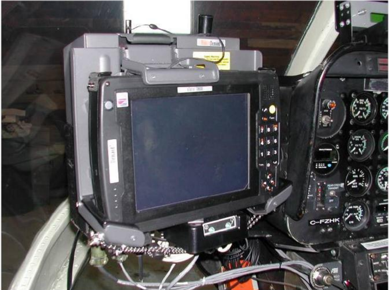
Photo 1: AGIS installed in the Bell 206
