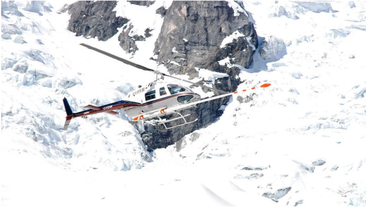
FIGURE 10: BELL 206 JET RANGER EQUIPPED IN STINGER CONFIGURATION FOR MAGNETIC DATA ACQUISITION
