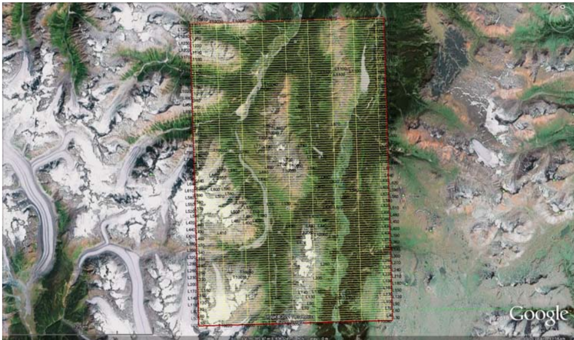
Figure 2: Survey and tie lines outlined in yellow and the boundary in red in plane view.
