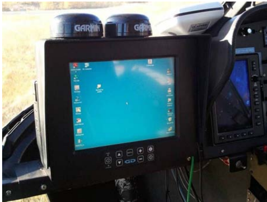
Figure 8: AGIS installed in the Eurocopter AS350.
