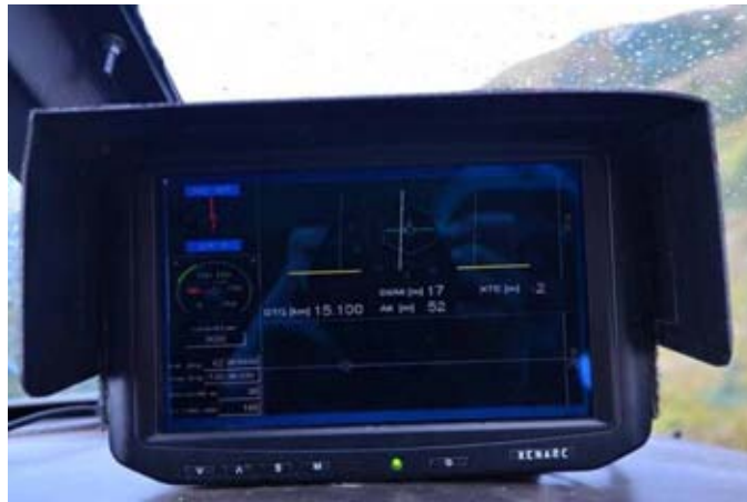
Figure 13: Pilot Guidance Unit.
