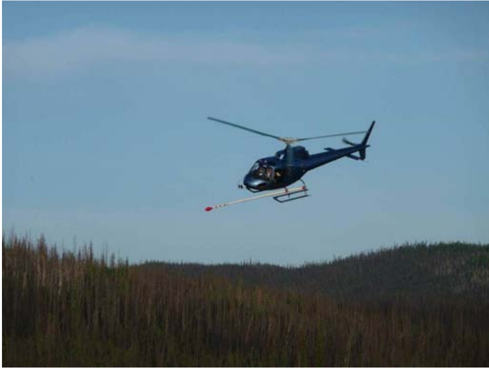
Figure 7: Eurocopter AS350 equipped with mag stinger for magnetic data acquisition.
