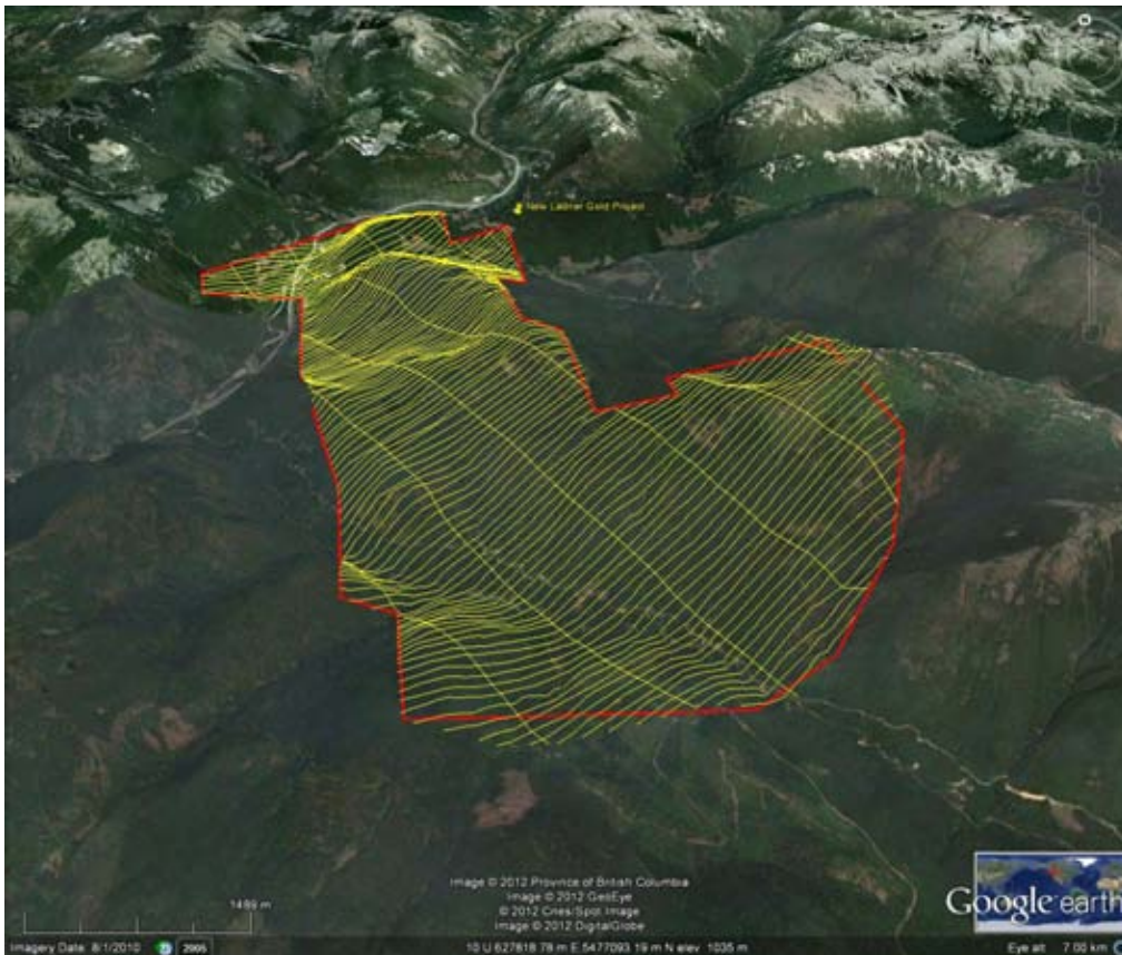
Figure 5: New Ladner Gold Project survey area with survey and tie lines shown in yellow and the boundary outlined in red in terrain view.
