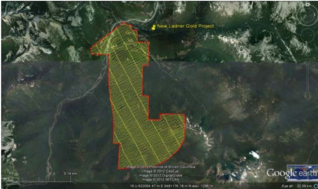
Figure 4: New Ladner Gold Project survey boundary with survey and tie lines shown in yellow and the boundary outlined in red in plane view.
