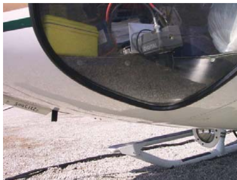
Figure 4. Digital video camera typical mounting location
