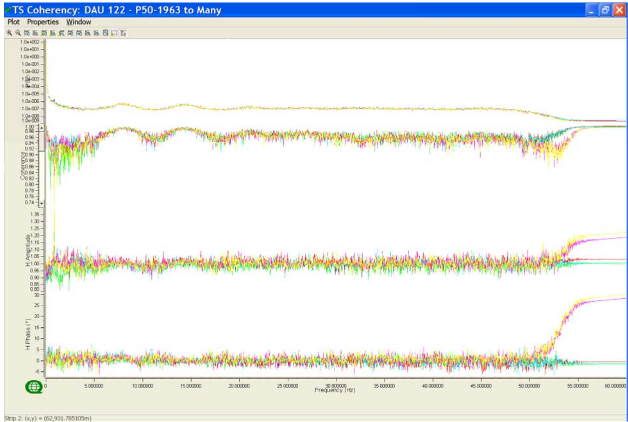
From top to bottom: PSD of channels and Coherency and Response Function (Amplitude and Phase) compared to Reference Channel – Linear frequency scale
