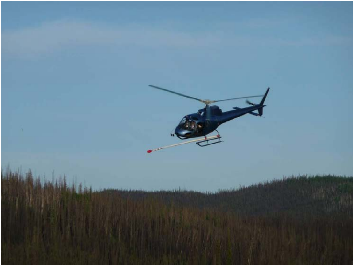
Figure 5: Eurocopter AS350 equipped with mag stinger for magnetic data acquisition.
