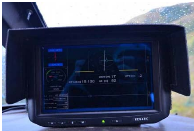
Figure 12: Pilot Guidance Unit.
