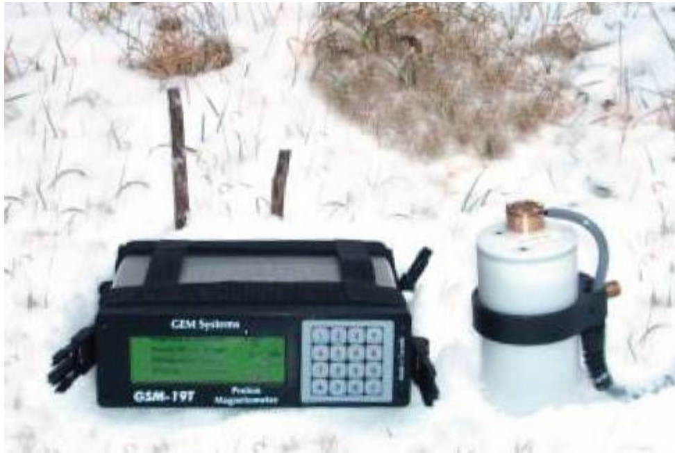
Figure 10: GEM GSM-19T proton precession magnetometer.
