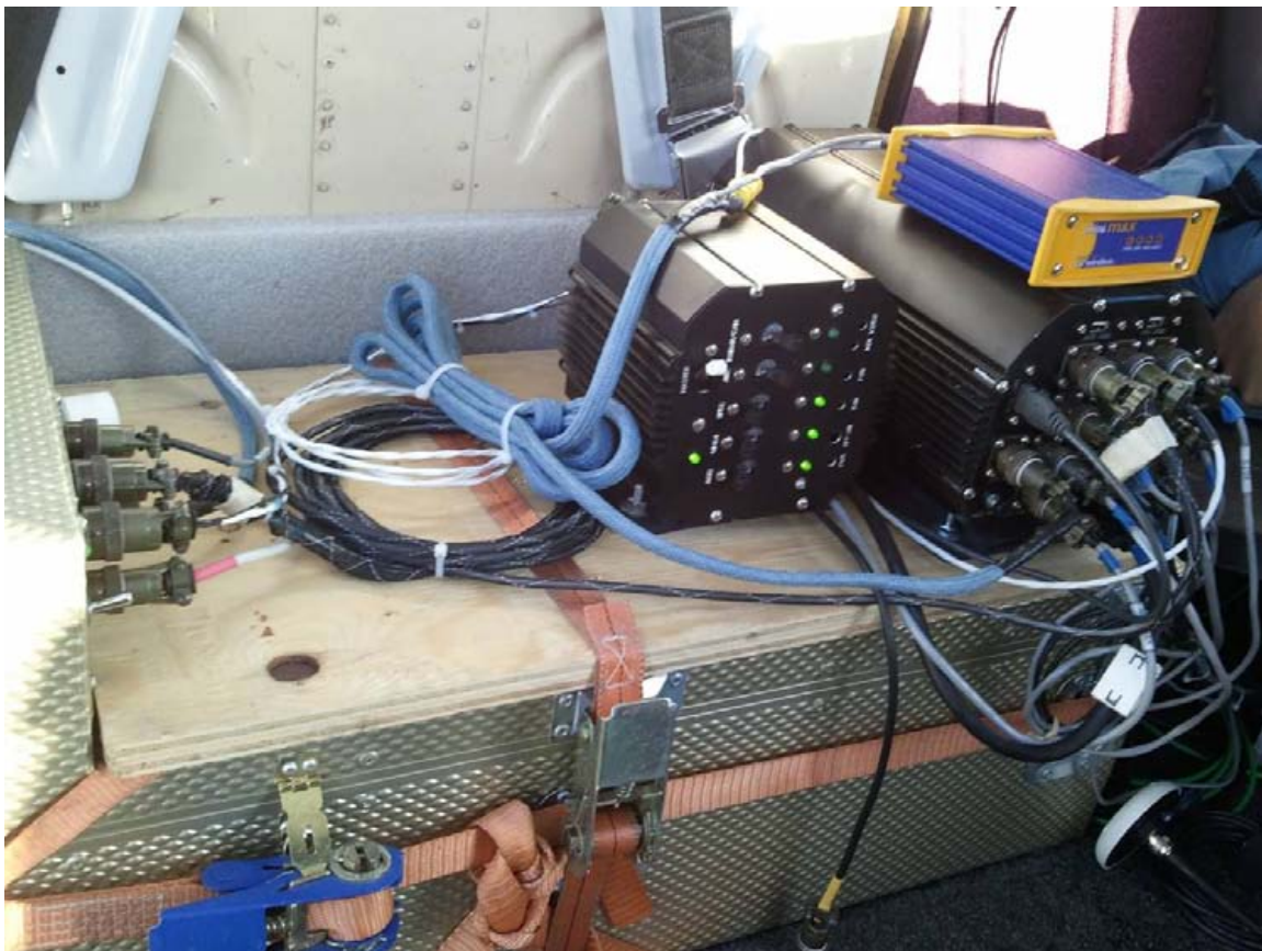
Figure 7: One of the IRIS strapped in the back seat of the Eurocopter AS350.
