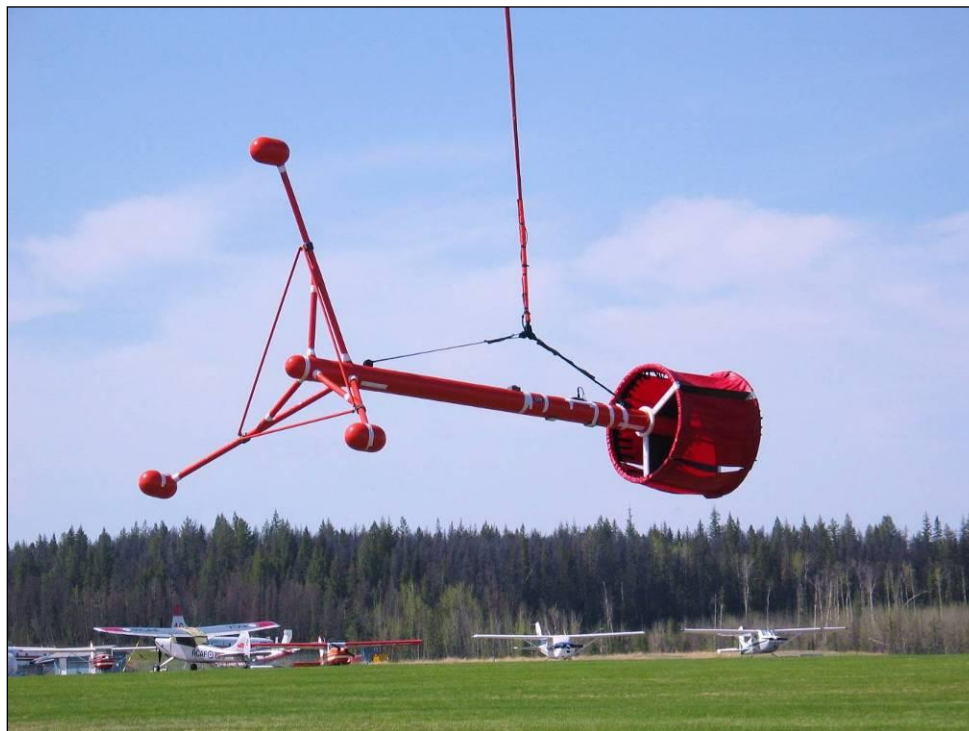
Figure 5 - The CMG tri-axial magnetic gradiometer.
