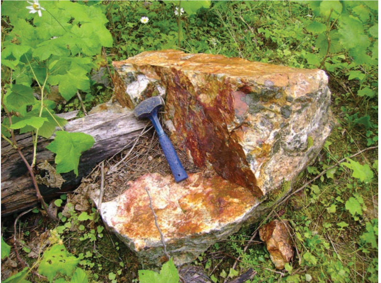
Plate 1: 1.53 g/t Gold and 265 g/t Silver Quartz Float in the V&M Mines Area
