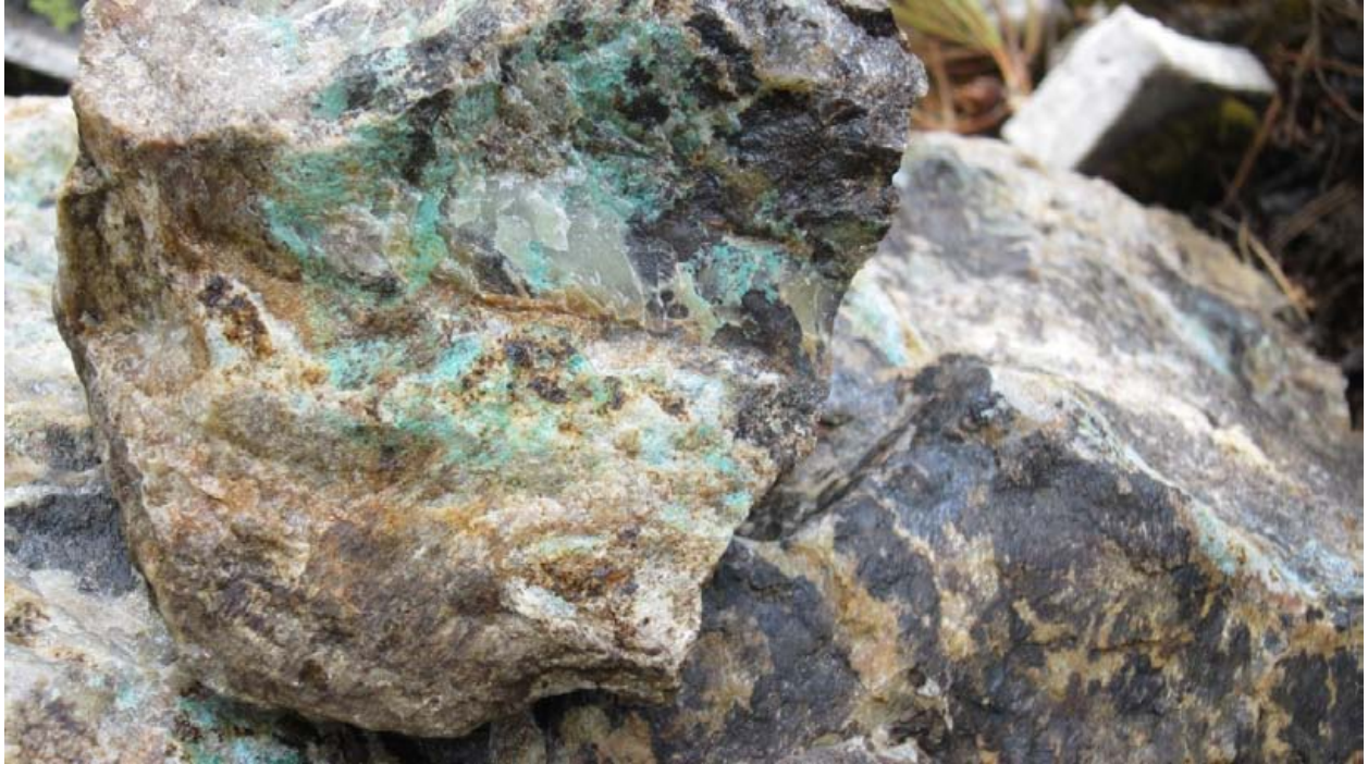
Photo 4: Mineralized quartzite, Jake Hill stratabound copper zone; note malachite, MnO 2 (pyrolusite?) and jarosite alteration.
