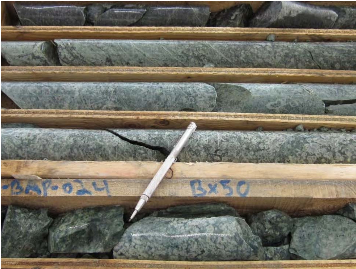
Figure 9-1: Drill core from hole 11BAP024, 185 m. The rocks are strongly serpentinized with relict pyroxene and olivine in a serpentine matrix.
