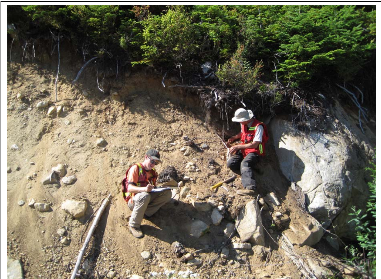
Photo 3: Minconsult field technicians gathering a soil sample. Colin Chudyk (left) and Richard Greenwood are pictured just above a logging road in a recent clear cut near the east boundary of the Ashlu Property. Note the thick sequence of glacial till containing mostly granitic boulders supported by silt and sand.
