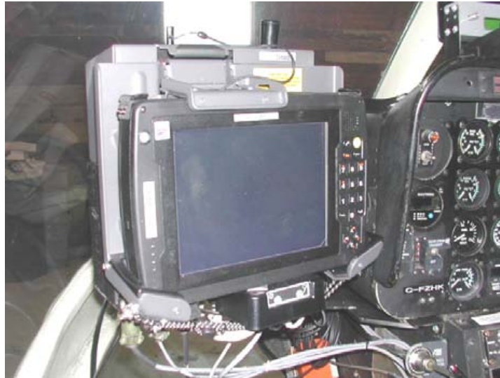
Figure 9: AGIS installed in the Bell 206.
