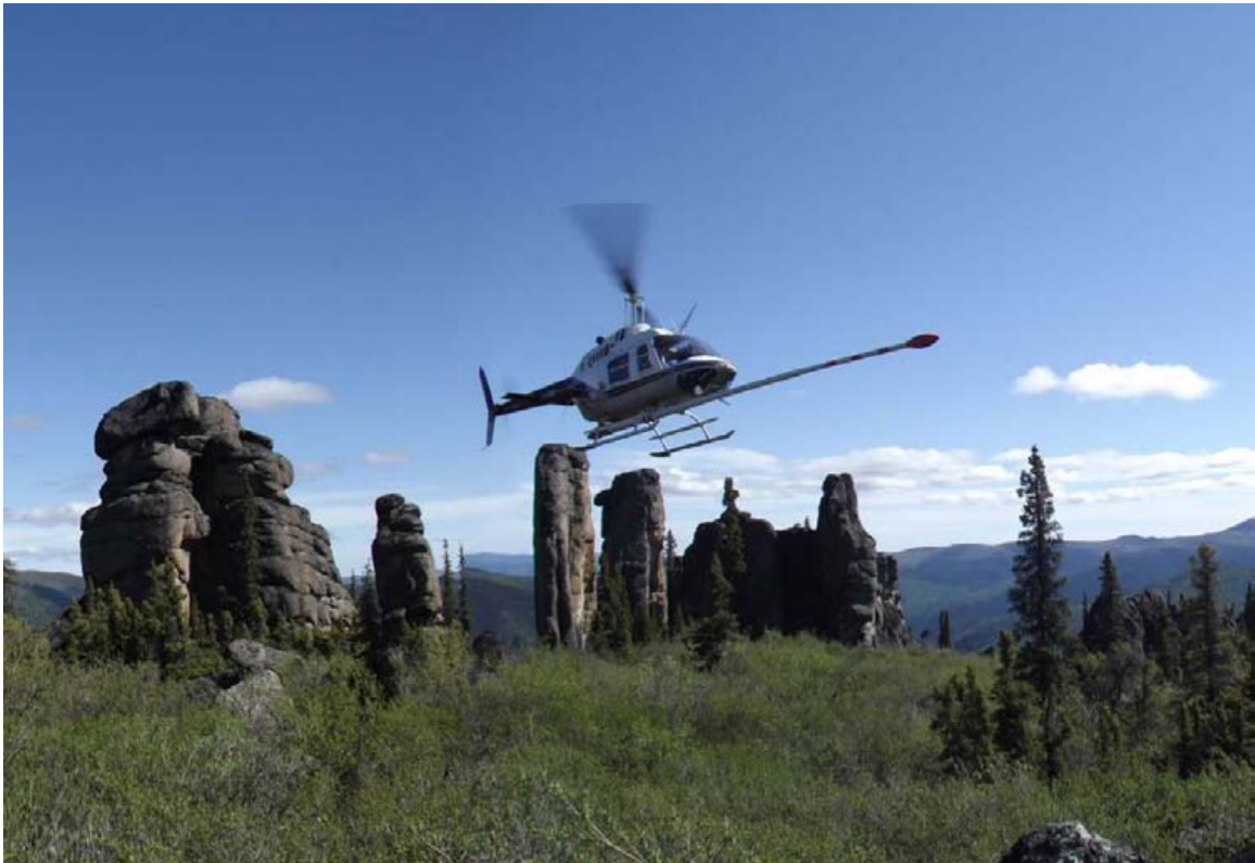
Figure 8: Bell 206 Jet Ranger equipped with mag stinger for magnetic data acquisition, and internal spectrometer crystals for radiometric data acquisition.
