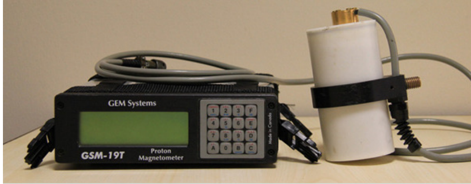
Figure 12: GEM GSM-19T proton precession magnetometer.
