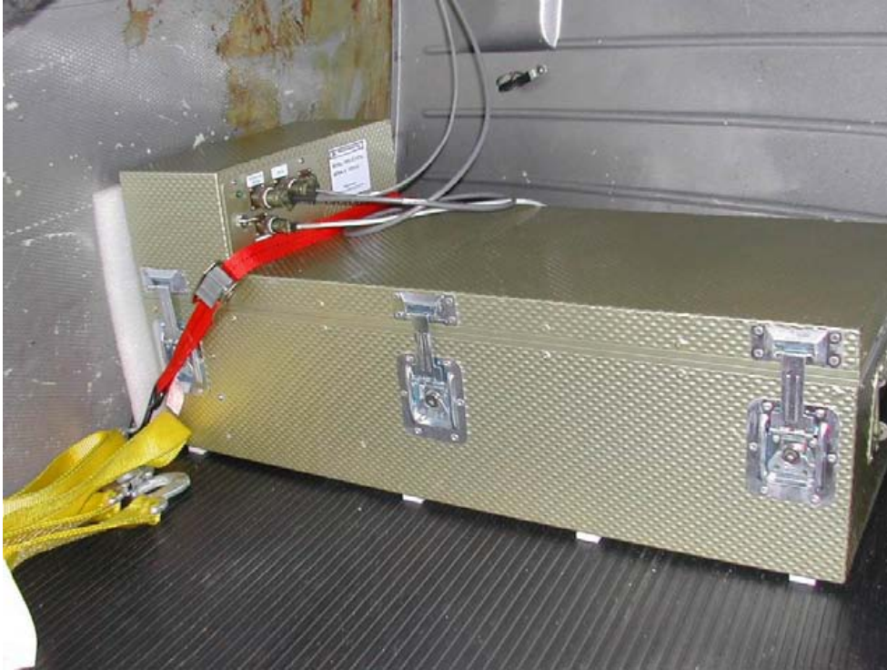
Figure 11: IRIS strapped into the cargo box of the helicopter.
